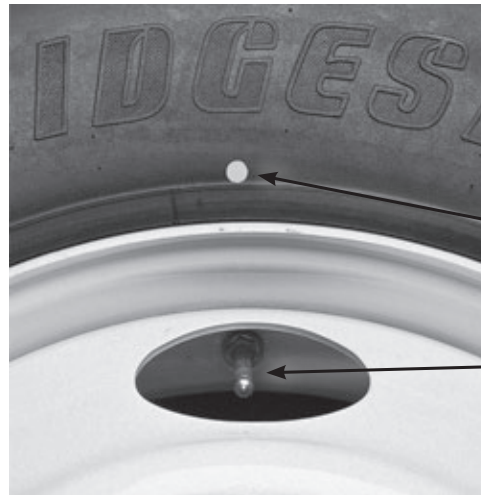
Tire light static balance mark (Yellow)
